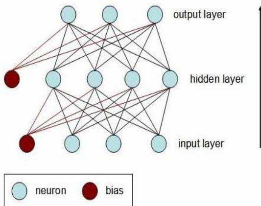
Fig. 1 Multilayer Perceptron Neural Network
