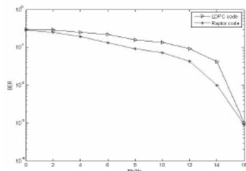
Fig.7: BER performance of Raptor and LDPC codes in Rayleigh channel with 224 burst errors
