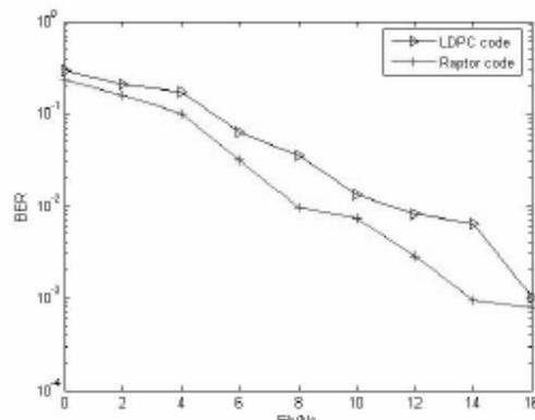
Fig.6: BER performance of Raptor and LDPC codes in Rayleigh channel with 80 burst errors
